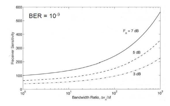
$N_p$  = 100 is realistic with a reasonable noise figure and filter bandwidth
